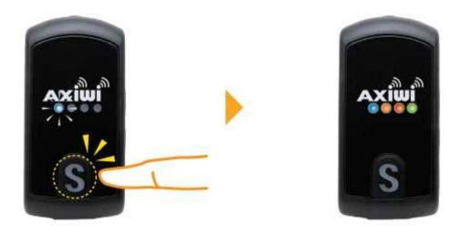
\* This function is to allow slave mode units to request the permission to speak. Permission is given on the first come first serve basis and maximum two slave mode units can get the permissions simultaneously.
