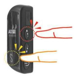
The channel LEDs will light up in turn by the order of channels. ((Blue -> Orange -> Red -> Green -> back to Blue -> etc.)
